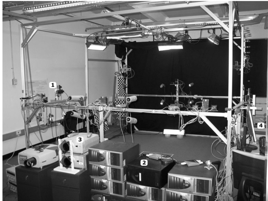
FIGURE 1 The tele-immersion system. Camera clusters (1) capture images of objects inside the cage. The computer array (2) processes the images to create a 360 degree representation. Dual projectors (3) project a polarized image to a projection screen (not shown.) The operator station (4) controls the system and provides the display for the review phase.
