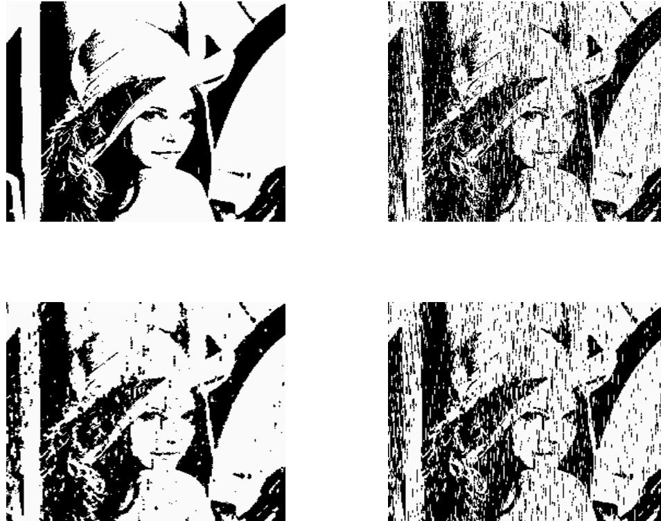
Figure 3: top-left : noiseless image; top-right : noisy image; bottom-left : denoised image by the proposed denoiser; bottom-right : denoised image by DUDE
