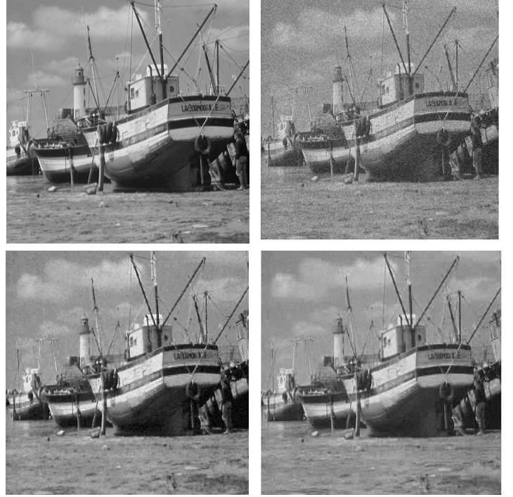
Fig. 3. Top-left: Original image, top-right: Noisy image (corrupted by an AWGN, \sigma = 15 ), bottom-left: Denoised image using the scheme in [2] ( 2k + 1 = 13 ) RMSE = 9.441, bottom right: Denoised image using the proposed scheme RMSE = 8.913 ( M = 10, 2k + 1 = 13 )
