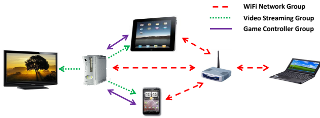
Figure 16: Coexistence in Dense Environments: Picasso enables devices operating in multiple networks to flexibly share fragmented spectrum and RF front ends, yet operate in a decoupled manner.
