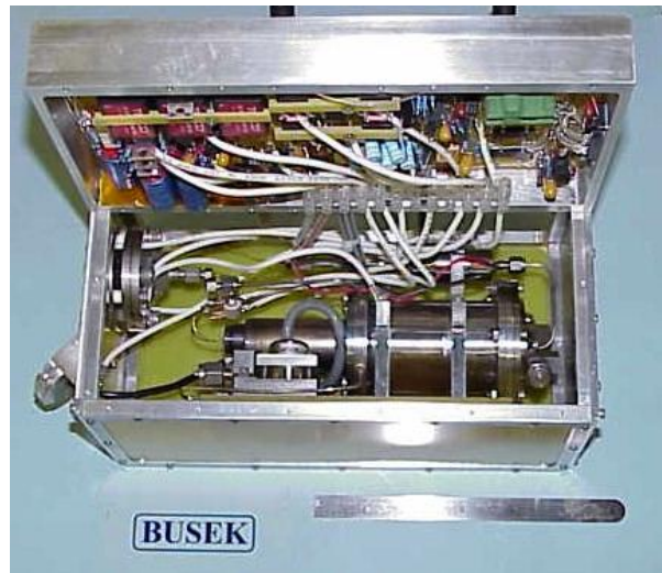
Figure 7 The 20- \mu N colloid thruster system during integration with the power-processing unit
