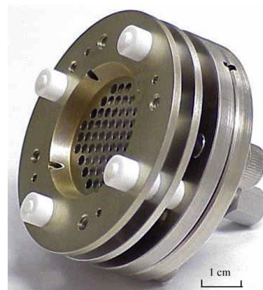
Figure 5 The 20- \mu\text{N} colloid thruster, which has 57 needles (nano droplet emitters), extractor grid, and an accelerator grid. The double grid is necessary to achieve the required thrust stability.
