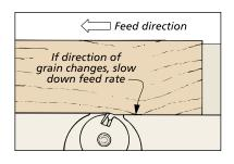
and joint the concave edge until you can "hear" the jointer cutting along the entire length of the piece.
