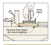
a jointer as an edge-cutting tool, it's also great for flattening a board's face. And the procedure is the same.
