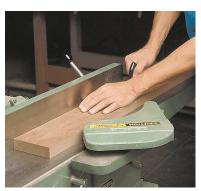
**Joint one face**. Flattening one face first is the key to ending up with pieces that are flat, straight, and square.
