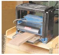
**Thicknessing the stock**. A planer not only reduces the thickness of the board. It creates a face that's flat and parallel to the jointed face.
