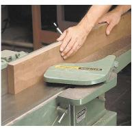
**Joint an edge**. Now that both faces are flat and parallel, you can begin to work on the edges. So it's back to the jointer to clean up one edge.
