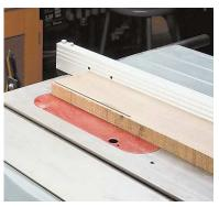
**Final edge**. To get the second edge straight and parallel with the first, it can be ripped on the table saw (and cleaned up on the jointer, if needed).
