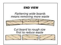
you have to remove more wood to get it flat. Take a cupped board for example. To joint and plane across its entire width means removing a lot of material at the center, as shown in the drawing. But if the board is ripped into narrow pieces first, there will be much less waste.
