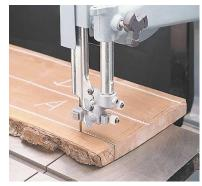
**Roughing it**. Cutting pieces to rough size first means there's less material to remove to get them flat and straight.
