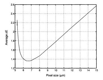
**Figure 7.** Average  $\Delta E$  versus pixel size
