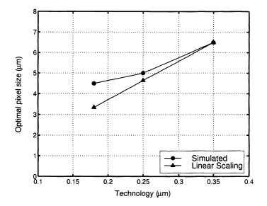
Figure 9. Optimal pixel size versus technology
