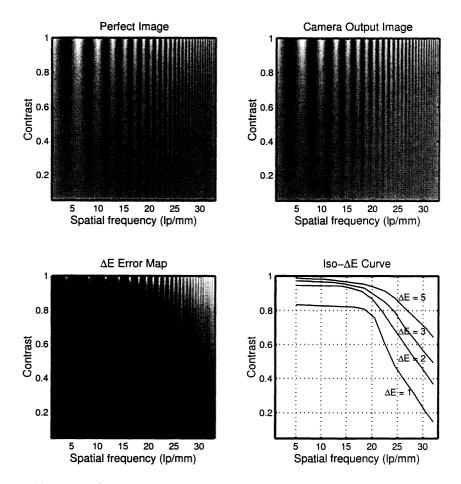
Figure 5. Simulation result for a  $0.35\mu$  process with pixel size of  $8\mu$ m
