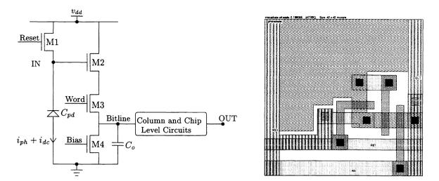
Figure 1. APS circuit and sample pixel layout
