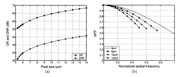
Figure 2. (a) DR and SNR (at 20% well capacity) as a function of pixel size. (b) Sensor MTF (with spatial frequency normalized to the Nyquist frequency for  $6\mu$ m pixel size) is plotted assuming different pixel sizes.
