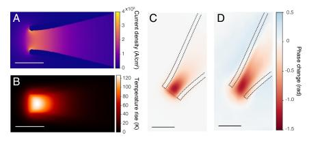
**Fig. 2.** QPI of Joule heating in electrolyte. (A) Density of electric currents delivered via a glass pipette of 6.4  $\mu$ m inner diameter (computational modeling). (B) Temperature at the end of the 20- $\mu$ s pulse. (C) Calculated phase change at the end of the heating pulse, with its maximum of -1.24 rad. (D) Experimental QPI map with a maximum phase change of -1.22 rad at the end of the electrical pulse. (Scale bars: 10  $\mu$ m.)
