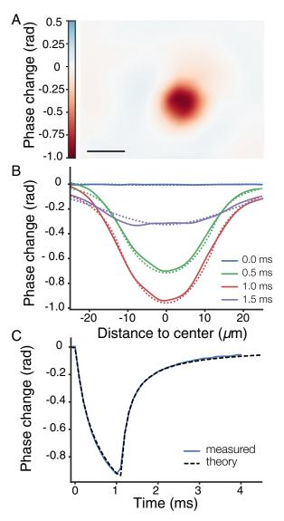
**Fig. 1.** QPI of the heating of a thin absorptive layer. (A) Phase change at the end of a 1.1-ms-long pulse of 11 mW peak power, focused into a 25- $\mu$ m spot on an absorptive film. (Scale bar: 25  $\mu$ m.) (B) Radial profile of the phase change at various time points (t = 0 is the beginning of the heating pulse). Solid lines, experimental measurements; dashed lines, computational modeling. (C) Phase signal in the center of the heating beam over time: experimental and computed data.
