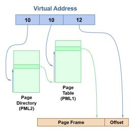
Each page table entry includes the following bits in addition to a physical page frame number: present, read-only, protected (only kernel can access), referenced, and dirty.
