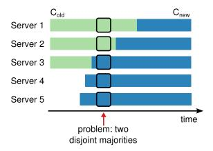
**Figure 4.2:** Switching directly from one configuration to another can be unsafe because different servers will switch at different times. In this example, the cluster grows from three servers to five. Unfortunately, there is a point in time where two different leaders can be elected for the same term, one with a majority of the old configuration ( $C_{\text{old}}$ ) and another with a majority of the new configuration ( $C_{\text{new}}$ ).
