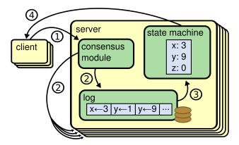
**Figure 2.1:** Replicated state machine architecture. The consensus algorithm manages a replicated log containing state machine commands from clients. The state machines process identical sequences of commands from the logs, so they produce the same outputs.
