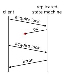
**Figure 6.2:** An example of an incorrect results that can arise from duplicated commands. A client submits a command to a replicated state machine to acquire a lock. The client's first command acquires the lock, but the client never receives the acknowledgment. When the client retries the request, it finds that the lock is already taken.
