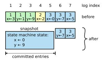
**Figure 5.2:** A server replaces the committed entries in its log (indexes 1 through 5) with a new snapshot, which stores just the current state (variables x and y in this example). Before discarding entries 1 though 5, Raft saves the snapshot's last included index (5) and term (3) to position the snapshot in the log preceding entry 6.
