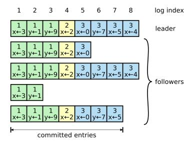
**Figure 3.5:** Logs are composed of entries, which are numbered sequentially. Each entry contains the term in which it was created (the number in each box) and a command for the state machine. An entry is considered *committed* if it is safe for that entry to be applied to state machines.
