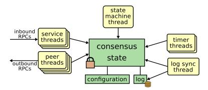
**Figure 10.1:** In LogCabin, consensus state for each server is stored in a monitor protected by a single lock, accessed by a collection of threads. The threads communicate with other servers ("peer threads"), handle incoming requests from clients and other servers ("service threads"), execute commands in the state machine ("state machine thread"), implement timeouts ("timer threads"), and write log entries to disk ("log sync thread").
