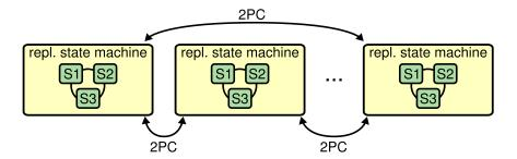
**Figure 2.3:** Partitioned large-scale storage system using consensus. For scale, data is partitioned across many replicated state machines. Operations that span partitions use a two-phase commit protocol.
