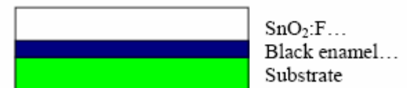
f) Solar-transmitting coating/blackbody-like absorber
