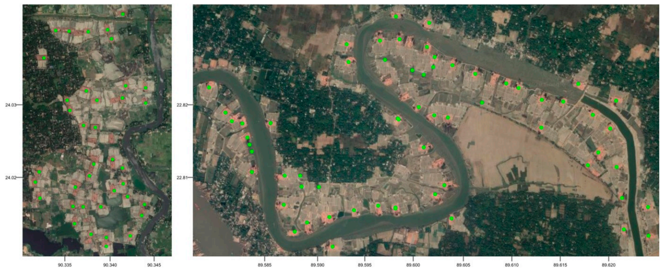
Fig. 2. Map of model-generated kiln coordinates. This map plots the coordinates identified by our model (shown in green) over satellite imagery for a cluster of kilns just north of Dhaka, near Gazipur, Bangladesh (Left) and Khulna District (Right). The kilns themselves are the red objects, which are surrounded by rows of drying bricks that appear as the brown color around each kiln.
