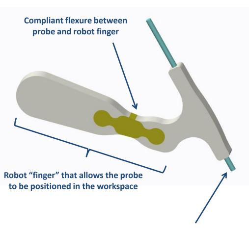
"Optical probe" (here just a 1.5 mm diameter glass fiber) embedded in the robot body
