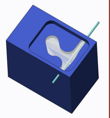
**[Left]** I chose to embed the fiber in the hard urethane by drilling a hole on the side of the mold. The fiber is inserted into this hole. By underdimensioning the hole (by about 50 microns), the machinable wax made a very tight seal around the fiber.
