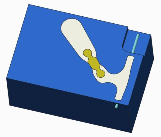
**[Top row]** Machining of the initial mold for hard urethane (Task 4). Optical fiber is held within the mold.
