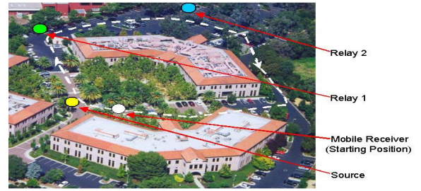
Fig. 1. Network Set-up for Multihop Routing Experiments. The receiver moves clockwise along the indicated trajectory
