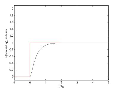
Here there is no overshoot at all and settling takes ~  $3\pi/\omega_0$ . Finally we consider the critically damped case,
