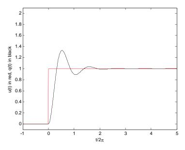
Here the overshoot is greatly reduced and the system settles within a time  $\sim 4\pi/\omega_0.$  Next the overdamped case,
