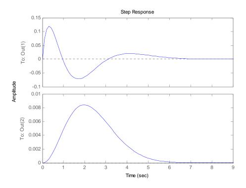
The response to a step in the disturbance torque  $T_d$  is obtained by  $motdrv = ss(A-B*K, [0;0;0;0.1], [0 \ 0 \ 1 \ 0;0 \ 0 \ 0 \ 1], []),$  step(motdrv),yielding
