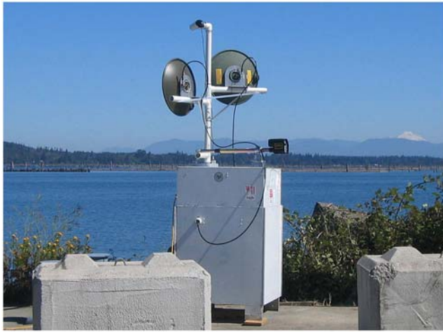
Figure 4. RiverRad, a pulsed Doppler X band radar built by the Applied Physics Laboratory, University of Washington, shown in operation on the bank of the Snohomish River at Everett, Washington. Its location is indicated by the black circle in Figure 2 at (558.61, 5318.6) km.
