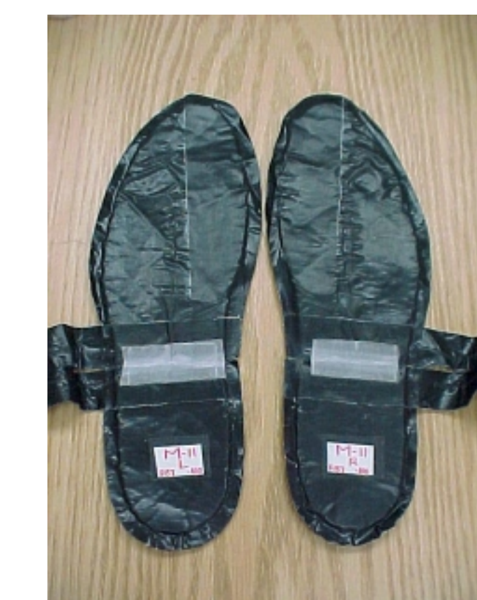
Elements of the vibro-tactile feedback system. Vibrators (left figure) are placed in contact with heel and toe of each foot. The foot-switches (middle figure) sense which foot is off the ground. The interface box (right figure) receives collision information from the computer system and provides a 250ms vibration cue to the heel or toe of the foot involved in a collision.
