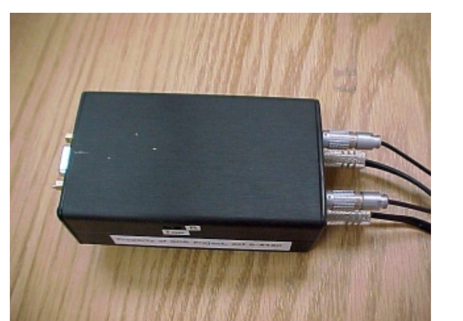
Elements of the vibro-tactile feedback system. Vibrators (left figure) are placed in contact with heel and toe of each foot. The foot-switches (middle figure) sense which foot is off the ground. The interface box (right figure) receives collision information from the computer system and provides a 250ms vibration cue to the heel or toe of the foot involved in a collision.
