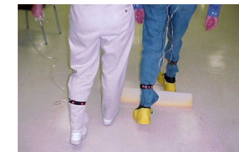
Subject (on right) stepping over a series of foam obstacles during an evaluation session. The LEDs on the subject indicate heel strike, while the LEDs on the therapist are lit when a collision is observed. All evaluation sessions are videotaped to provide timing information.
