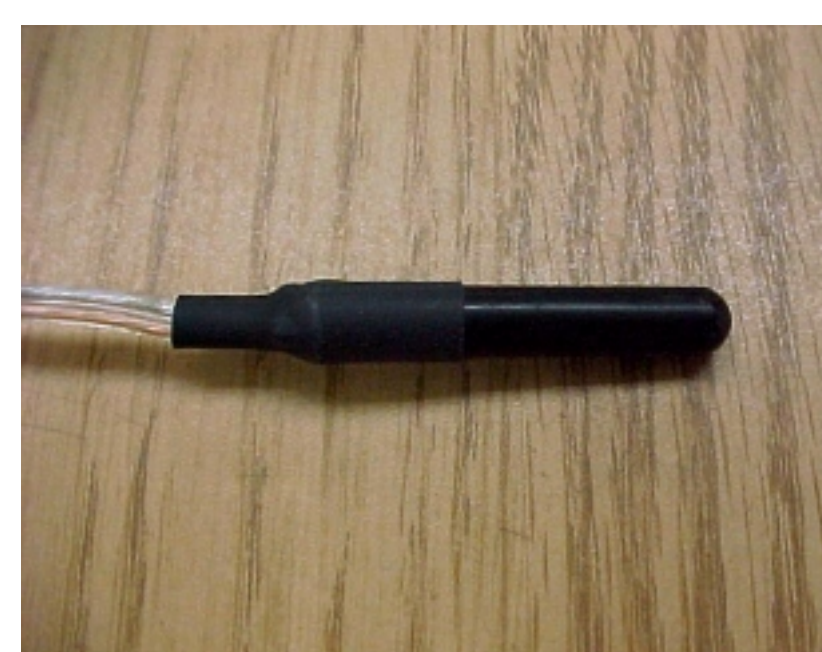
Elements of the vibro-tactile feedback system. Vibrators (left figure) are placed in contact with heel and toe of each foot. The foot-switches (middle figure) sense which foot is off the ground. The interface box (right figure) receives collision information from the computer system and provides a 250ms vibration cue to the heel or toe of the foot involved in a collision.
