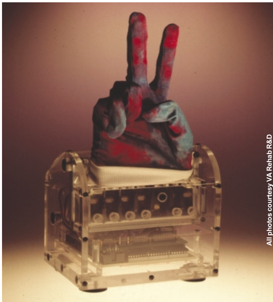
Ralph the fingerspelling hand: an electromechanical hand that signs letters according to the American One-Hand Manual Alphabet (a special form of sign language). This device aids deaf-blind users and can accept and sign data from multiple sources such as a computer, a voice recognition system, or a closed caption television decoder.
