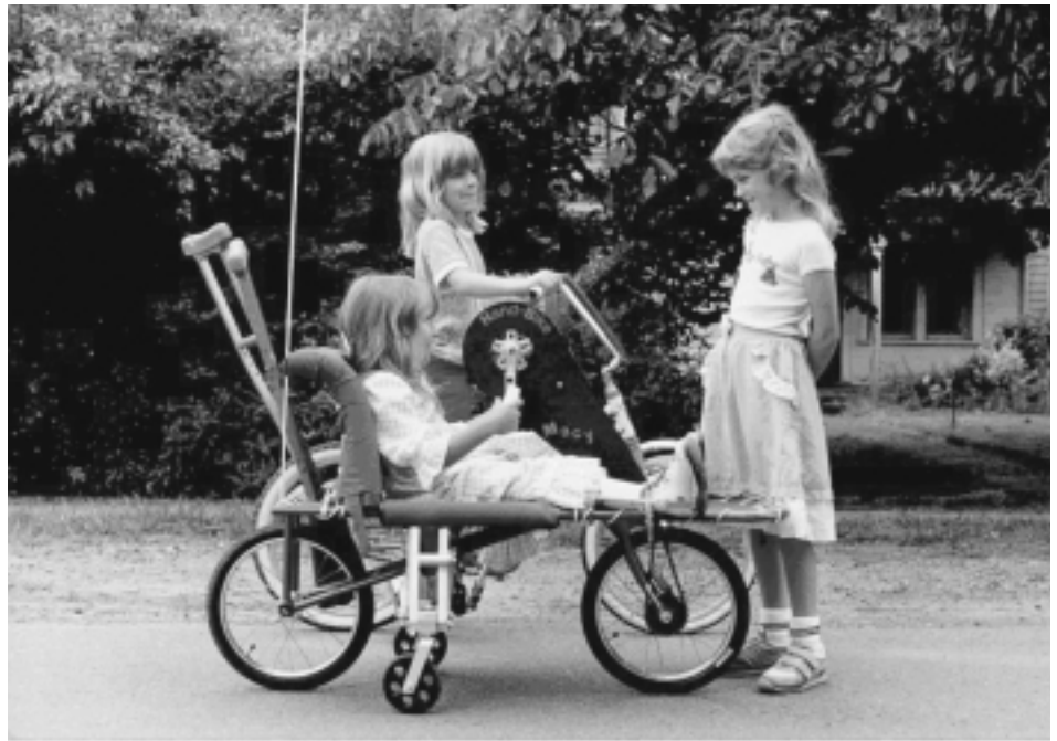
[Above] Handbike: an arm-powered, two-wheeled bicycle designed for people with lower limb disabilities. Two smaller wheels automatically touch down and prevent the bike from leaning over too much or from falling over.
