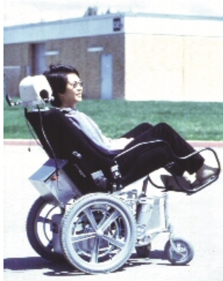
[Above] Ultrasonic Head Controlled Wheelchair Interface: a device that allows quadriplegics to wirelessly control their wheelchair. It is used similarly to a joystick: tilting the head forward moves the wheelchair forward, tilting left, right, or backwards moves the wheelchair in that respective direction.
