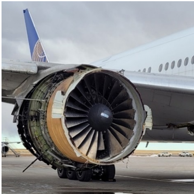
PW4077 fan front view – Denver accident
