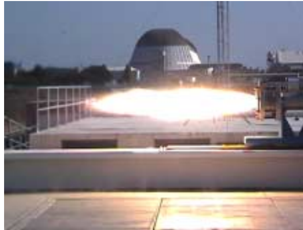
Figure 11.10 Hybrid motor test at NASA Ames. Thrust is approximately 2500 pounds with a simple convergent nozzle.
