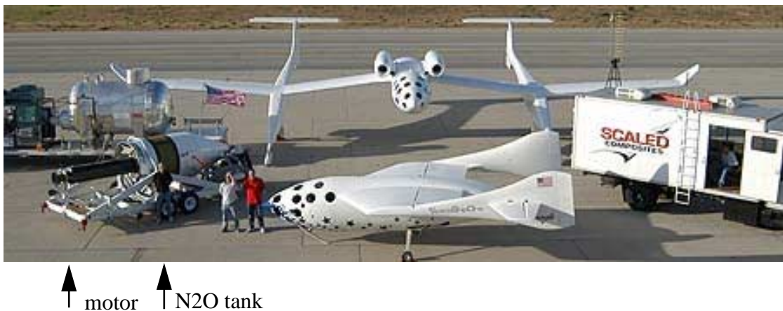
Figure 11.8 Various systems of Space Ship One. Note the hybrid rocket on the left.
