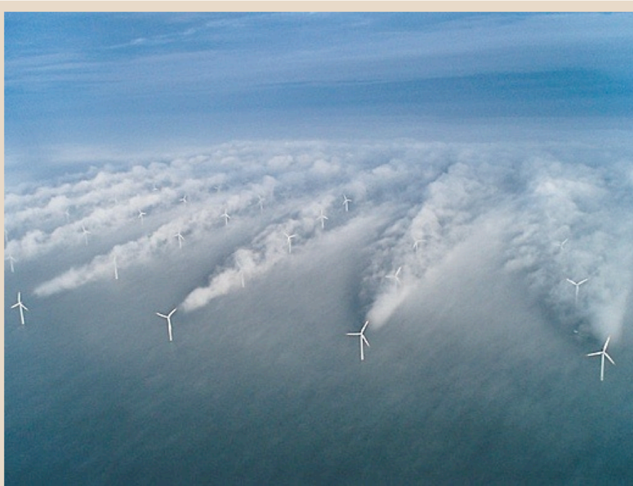
Image above: The above photograph shows the turbulence field behind the Horns Rev offshore wind turbines. Horns Rev is located in the North Sea, 14 kilometers west of Denmark. Photographer Christian Steiness. From ( http://wattsupwiththat.com/2011/04/28/the-wind-turbine-albedo-effect/ ).
