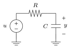
current flowing into capacitor is  $Cy'(t) = \frac{u(t) - y(t)}{R}$
