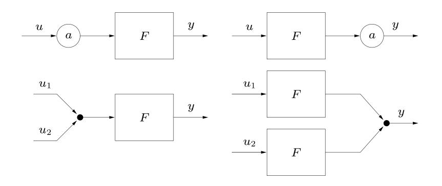
**examples of linear systems:** scaling system, differentiator, integrator, running average, time shift, convolution, summer, difference systems
