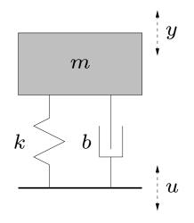
(can represent suspension system, building during earthquake, . . . )
