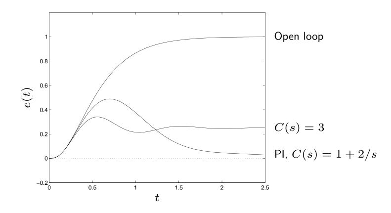
note that the temperature error  $\boldsymbol{e}$  converges to zero
