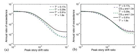
Figure 7. Risk-based assessments of *PSDR* of the four-story perimeter frame (Building No.1008) obtained from ground motions with (a) approximate CS with approximate conditional standard deviations and (b) refined CS with inflated conditional standard deviations.
