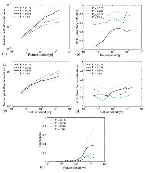
Figure 8. Statistics of structural responses from intensity-based assessments of the four-story perimeter frame (Building No.1008) using the CS (a) median *PSDR*, (b) logarithmic standard deviation of *PSDR*, (c) median *PFA*, (d) logarithmic standard deviation of *PFA*, and (e) probability of collapse.
