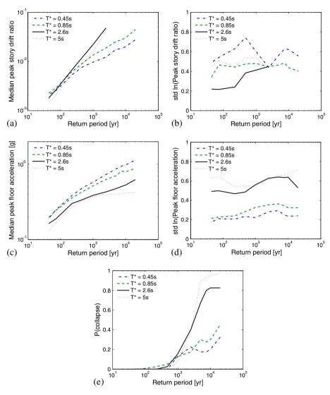
Figure 1. Statistics of structural responses from intensity-based assessments of the 20-story perimeter frame (Building No.1020) using the CS (a) median *PSDR*, (b) logarithmic standard deviation of *PSDR*, (c) median *PFA*, (d) logarithmic standard deviation of *PFA*, and (e) probability of collapse.
