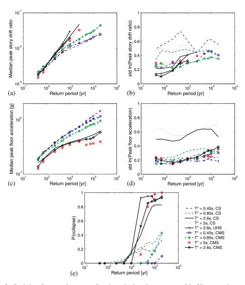
Figure 3. Statistics of structural responses from intensity-based assessments of the 20-story perimeter frame (Building No.1020) (a) median *PSDR*, (b) logarithmic standard deviation of *PSDR*, (c) median *PFA*, (d) logarithmic standard deviation of *PFA*, and (e) probability of collapse.
