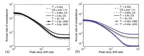
Figure 4. Risk-based assessments of *PSDR* of the 20-story perimeter frame (Building No.1020) obtained from ground motions selected to match the CS (all four conditioning periods) as well as the CMS and the UHS for (a)  $T^* = 2.6$  s and (b)  $T^* = 0.45$  s.
