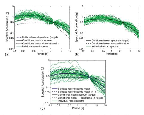
Figure 2. Response spectra of selected ground motions with (a) UHS, (b) CMS, and (c) CS as target spectra for Sa(2.6 s) associated with 2% in 50 years probability of exceedance for the 20-story perimeter frame (Building No.1020).
