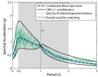
Figure 10. CMS (with  $T^*=1s$ ), the CMS +/- the conditional standard deviation from equation 11, and the response spectra from ground motions selected previously to match the CMS.
