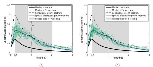
Figure 8. Conditional mean spectrum for the Riverside example site (with  $T^{*=1s}$ ), and response spectra from ground motions selected to match this target spectrum. (a) Ground motions selected after scaling spectra to match the target  $Sa(T^*)$ . (b) Ground motions selected after scaling spectra to match the CMS over the entire period range considered.
