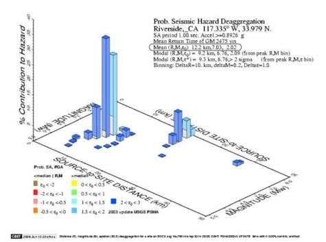
Figure 2. PSHA deaggregation for Riverside, given *Sa*(1s)>0.89g. (Figure from USGS Custom Mapping and Analysis Tools, <u>http://earthquake.usgs.gov/research/hazmaps/interactive/</u>, 2008. Emphasis on mean deaggregation values added by the author.)
