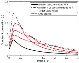
Figure 9. Conditional Mean Spectra, conditioned on *Sa* values at several periods, but having an equal probability of exceedance.
