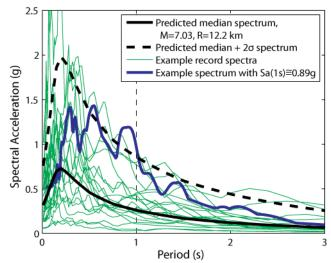
Figure 4. Response spectra from real ground motions having approximately magnitude = 7 and distance = 12 km. The example spectrum shown with a heavier line is the Castaic Old Ridge Route recording from the M = 6.7 Northridge earthquake, recorded on a Class C site with a closest distance to the fault rupture of 20 km.
