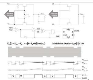
Figure 17.6.4: Demodulator schematic along with the description of the asynchronous pulse-width ASK modulation. The equation describes amplitude modulation, with modulation depth as defined.
