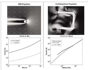
Figure 17.6.2: Performance summary of the electromagnetic propulsion mechanisms determined with numerical fluid simulations.
