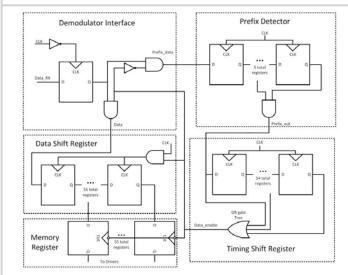
Figure 17.6.5: Digital controller schematic depicting the operation of the data receive circuitry.
