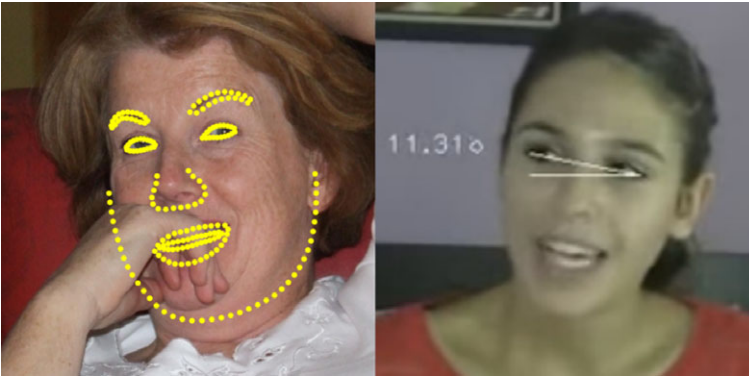
Figure 1: Left, shape-fitting output from Kazemi and Sullivan (2014), showing robustness to occlusion. Right, visualization of our adaptation for the calculation of head cant angle on a vlog from our dataset, calculated by first fitting a shape model of the face to find landmark points as on the left, and then triangulating cant angle from the corners of the eyes
