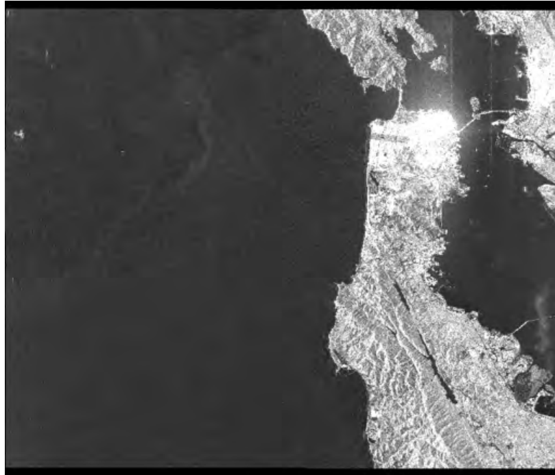
Figure 2.5: A sample SAR image of San Francisco, taken by ALOS on MAR 25, 2011. San Francisco and Oakland urban areas, dominated by corner reflectors, appear to be the brightest, while the Pacific Ocean, belonging to flat surfaces, appears to be darkest in the SAR image.
