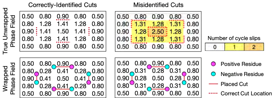
Figure 5.2: Simple examples of high-gradient accommodation in SNAPHU. In the left example, minimization of the length of cuts connecting positive and negative residues leads to the correct unwrapped solution. Minimization of the cuts connecting residues in the right example leads to a misidentification of cut locations and the first cycle slip. The center, fully-closed high-gradient loop in the right example has no residues, thus the algorithm does not correctly unwrap the phase at that location either, and the cycle slips accumulate to two.
