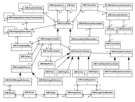
Figure 1 - AIM UML Class Diagram
