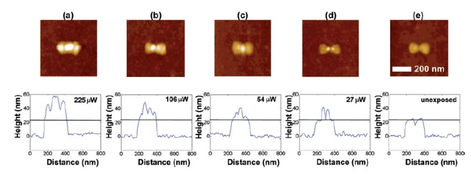
• The optical near-field of bowtie nanoantennas was used to achieve <u>local</u> twophoton photo-polymerization of SU-8 photoresist by pumping with an infrared modelocked laser
