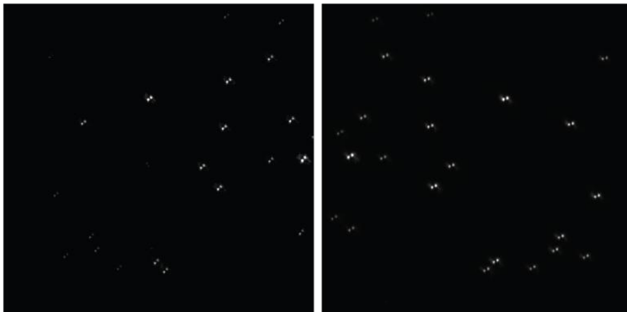
Figure 9. Example still image of beads on a coverslip during a control point scan. Still image of a field of view of fluorescent beads in the green (left) and red (right) channels during a control point scan.
