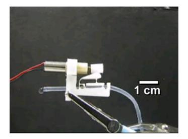
**S2.** Video of the motor actuated version of the peristaltic pump (video uploaded as a separate file). This pump operates at 3 V, with minimal back pressure, pumping deionized water. Figures of merit for the pump: operating voltage, 1.75 - 3 V; flow rate range,  $0 - 780 \mu$ /min; operating pressure 0 - 48 kPa; power consumption, 40 - 90 mW; weight, 3.6 g; package volume 6.2 cm<sup>3</sup>.
