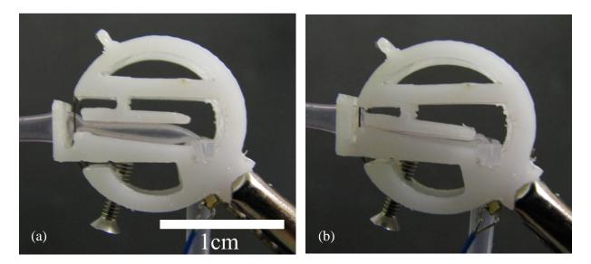
**S4.** (a) The SMA wire is relaxed (stretched): the upstream valve and pump chamber are both open and the pumping chamber refills from the upstream. (b) The SMA wire is contracted (electrical current is applied to the wire): the plunger closes the upstream valve and compresses the pumping chamber, raising the pressure within. This opens the downstream burst valve, and expels the fluid.
