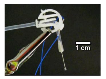
**S5.** Video of the SMA wire actuated version of the peristaltic pump (video uploaded as a separate file). This pump operates at 4 V, with minimal back pressure, pumping deionized water. Figures of merit for the pump: operating voltage, 4 V; flow rate range,  $0 - 60 \mu$ l/min; operating pressure, 0 - 69 kPa; power consumption, 420 mW; weight, 0.9 g; package volume 1.3 cm<sup>3</sup>.
