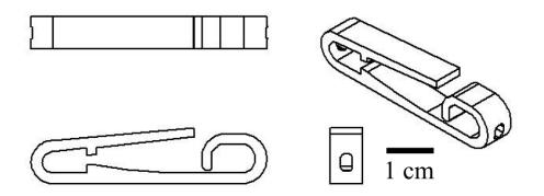
**S6.** Front, top, right, and isometric views (to scale) of the manually actuated version of the peristaltic pump. Drawings to scale.
