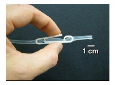
**S7.** Video of the manually actuated version of the peristaltic pump (video uploaded as a separate file). The pump is actuated by hand at several speeds and pumps deionized water with minimal back pressure. Faster actuation leads to larger flow rates. The pump weighs 2.6 g, and has a package volume of  $4.2 \text{ cm}^3$ .
