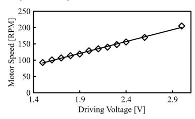
**S9.** Motor speed as a function of driving voltage while pumping deionized water at 22°C against minimal back pressure. As expected, motor speed (actuation frequency) increases linearly with driving voltage.
