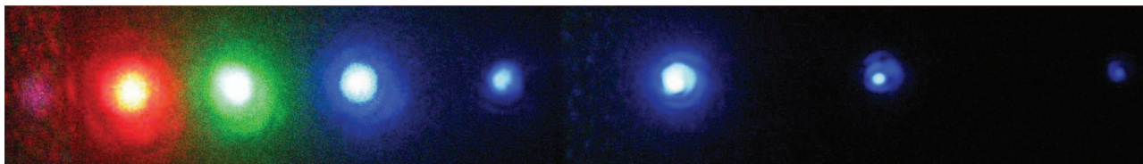
Fig. 4. Spatial modes of generated sidebands projected onto a white screen. Sideband wavelengths from left to right are 807 (faint), 650, 544, 488, 410, 365, 330, and 300 nm. The 650, 544, 488, and 410 nm beams have been attenuated by a factor of 10 with a neutral-density filter.
