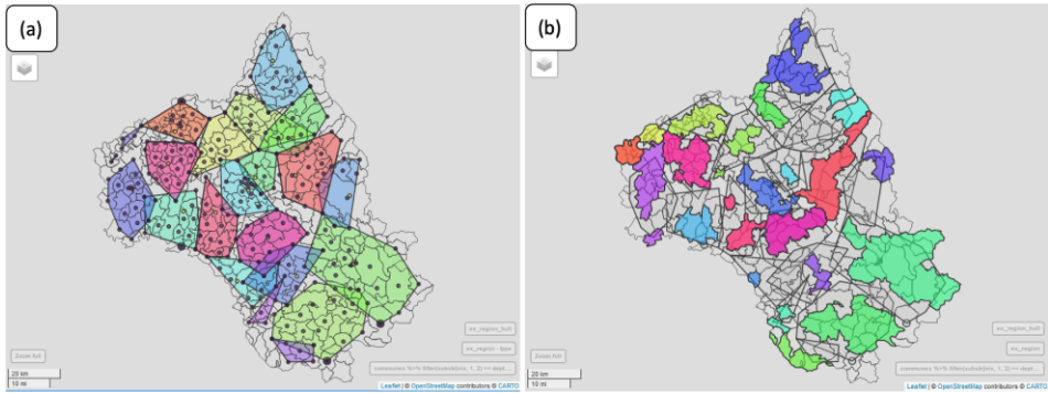
FIGURE A.6. Panel (a): convex hulls for the Aveyron department. Panel (b): (sub)counties that intersect with a single convex hull and the corresponding service territory of the substations (outcome of step 1).
