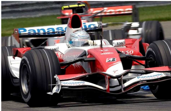
Figure: Rear-view mirrors are on the car body in the vicinity of the cockpit
