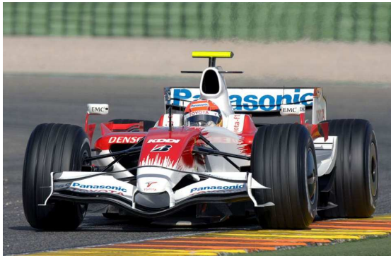
Figure: Rear-view mirrors are on sticks in the wake of the tires
