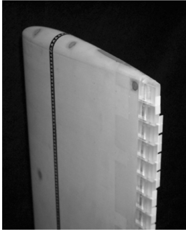
Fig. 2.7. A rear oblique view of the fully-assembled wing equipped with MiTEs.
