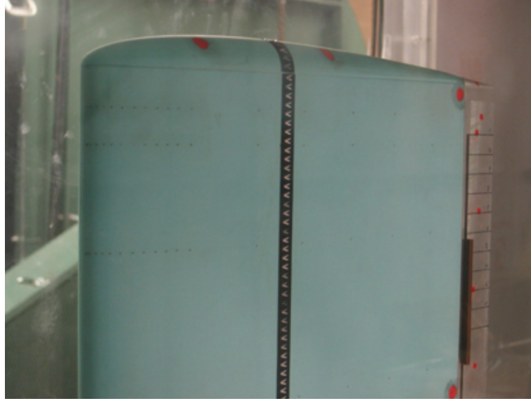
Fig. 5.6. The wing and spanwise actuating Gurney flap assembled and mounted in the wind tunnel.
