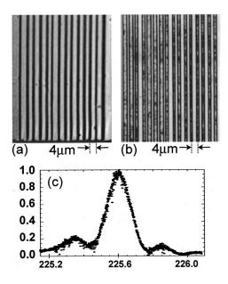
FIG. 2. 4-µm-period domains in backswitch poled 0.5-mm-thick LiNbO<sub>3</sub> substrate: (a) **y** surface; and (b)  $z^-$  surface view. Temperature-dependent phase matching for 460 nm SHG is shown in (c).
