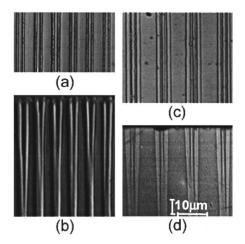
FIG. 3. Spatial frequency multiplication of domain structures by backswitch poling in 0.5-mm-thick LiNbO<sub>3</sub> having 10- $\mu$ m-period 2- $\mu$ m-wide patterned electrodes. Spatial frequency doubling: (a)  $z^+$  surface; and (b) y surface view. Spatial frequency tripling: (c)  $z^+$  surface; and (d) y surface view. In (d), the higher magnification in the x direction was obtained by using a tilted cross section.
