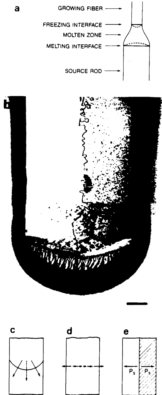
Fig. 11. Analysis of the temperature gradient and prediction of the domain structure in the a -axis grown fiber: (a) sketch of growth interface seen during growth; (b) grown-in interface seen on y -face, also shows the bi-domain structures of the a -axis fiber; (c) actual temperature gradient at the growth interface; (d) projection of the temperature gradient on the c -axis near the growth interface; (e) prediction of domain
