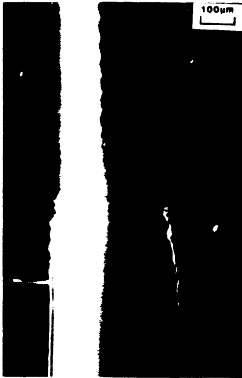
Fig. 6. Rotation of the three growth ridges by 60° can be seen at the seed-fiber interface of this c -axis grown fiber. This behavior is only seen when the - c -axis of the seed faces the melt.
