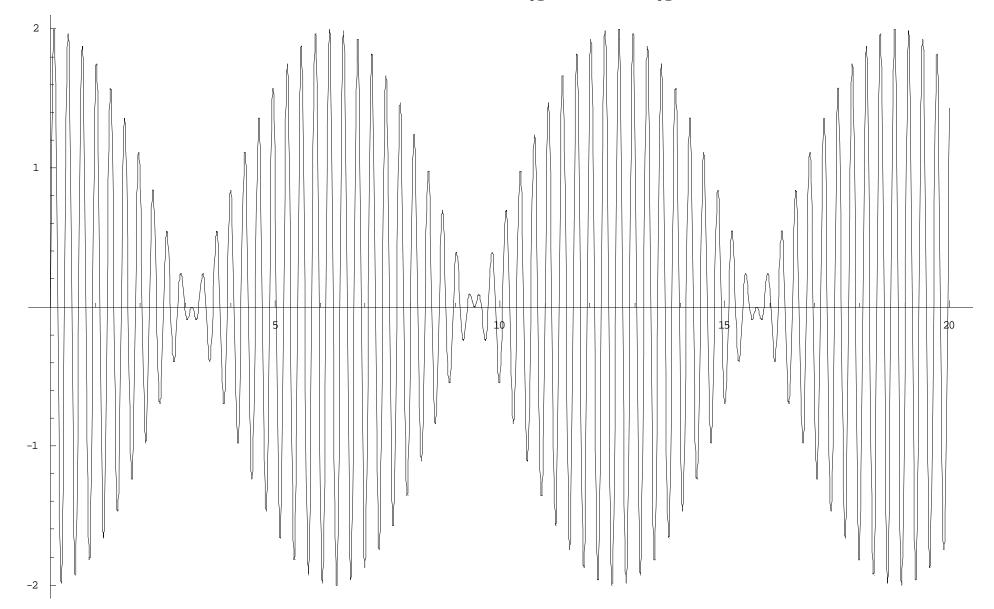
Amplitudes 2:1 – not 100% modulation ,  $\omega_{01} = 20.5$ ;  $\omega_{01} = 19.5$
