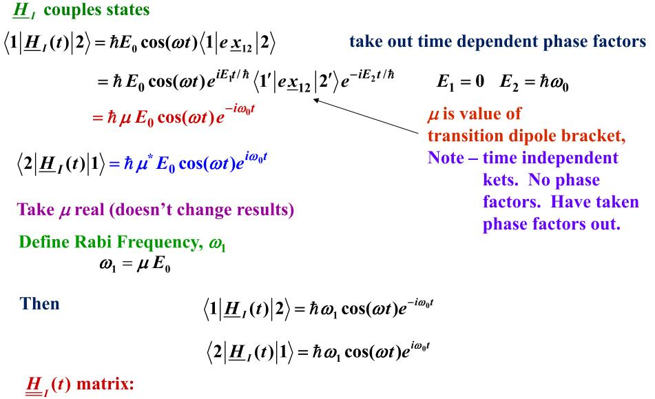
$$\underline{\underline{H}}_{I}(t) = \hbar \begin{bmatrix} 0 & \omega_{1} \cos(\omega t) e^{-i\omega_{0}t} \\ \omega_{1} \cos(\omega t) e^{i\omega_{0}t} & 0 \end{bmatrix}$$
