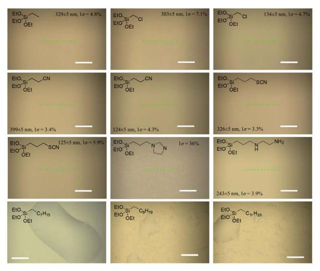
**Figure S6:** Results of spin coating BmimNTf<sub>2</sub> on substrates functionalized with triethoxysilanes with different head groups. The chemical used in functionalization is shown on each figure. After spin coating, if the IL forms a film, Raman spectra are measured at the green dots, and the variation of the N-S stretch in the  $NTf_2^-$  Raman signal is shown on the figure. White bars have lengths of 100  $\mu$ m.
