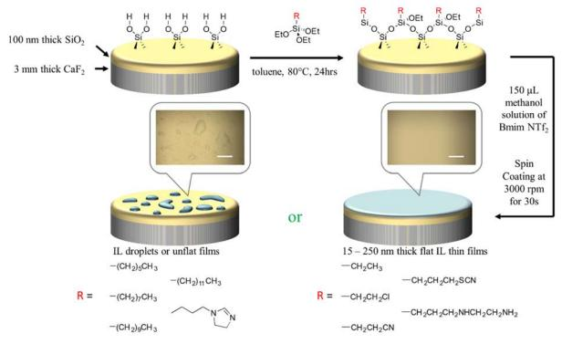
Figure S3: Surface functionalization and attempts to make ionic liquid thin films on neutral substrates.
