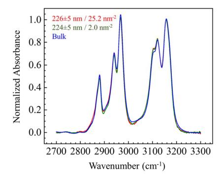
**Figure S7:** Normalized FT-IR spectra showing C-H stretching region of bulk IL and IL films. The film thickness and the surface charge density of the substrate are given in the figure. The spectra are the same within experimental error. Of particular importance is that the peak position are identical.
