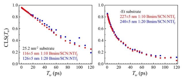
**Figure S2:** Comparison of CLS decays measured with 1:10 and 1:20 mixture of BmimSCN and BmimNTf<sub>2</sub> in ~120 nm films on a 25.2 nm<sup>-2</sup> charge density substrate (left) and ~220 nm films on a –Et substrate (right).
