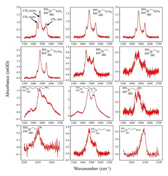
Figure S4. FT-IR spectra of functionalized neutral windows. The chemicals that were used for the functionalization reactions are shown in each graph.
