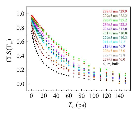
**Figure S1.**  $CLS(T_w)$  of ~220 nm IL films on different substrates. The inset shows the thicknesses of films, and the surface charge density on the substrate (in nm<sup>-2</sup>).
