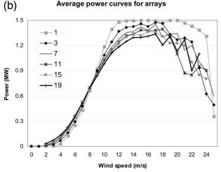
FIG. 7. (a) Cumulative frequency distribution and (b) wind power curve (MW) as a function of wind speed (m s<sup>-1</sup>), obtained after an array average.
