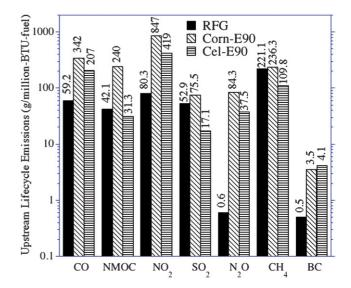
Fig. 3 Upstream lifecycle emissions of several individual pollutants from corn-E90 and cellulosic-E90 relative to reformulated gasoline (RFG).58
