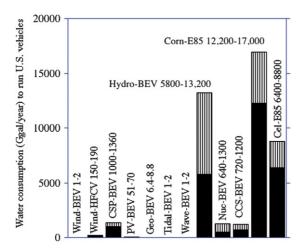
Fig. 7 Low (solid) and high (solid+lines) estimates of water consumption (Gigagallons year-1) required to replace all US onroad vehicles with other vehicle technologies. Consumption is net loss of water from water supply. Data for the figure are derived in ESI†. For comparison, the total US water consumption in 2000 was 148 900 Ggal yr<sup>-1</sup>.87
