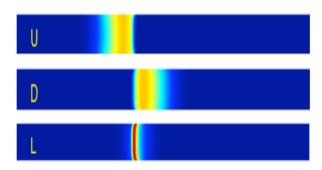
Mean concentrations of proteins U, L, and dye D at t=0.12~s. U and D just met and L is produced at their interface. The values of the contour levels go linearly from 0 (blue) to 1.3e-4 (red) mol/l
