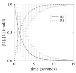
Time evolution of U and L concentrations in a homogeneous protein labeling reaction. The uncertainty in these concentrations, due to a 1% uncertainty in the labeling reaction rate parameters, is indicated by 63s "error bars."
