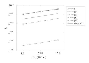
L2 norm of the difference between solutions on successive grids as a function of the fine grid spacing dxf. The slope of the lines shows a second-order spatial convergence rate for various species concentrations as well as the streamwise velocity.
