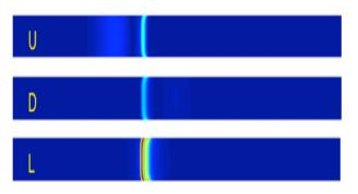
Standard deviation of the protein and dye concentrations at t=0.12 s. The values of the contour levels go linearly from 0 (blue) to 1.1e-5 mol/l (red). The largest uncertainties are found in the reaction zone.
