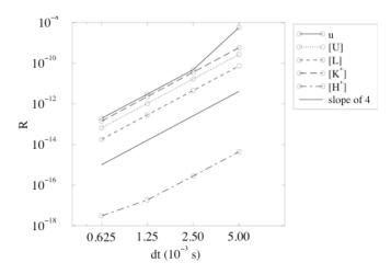
L2 norm of the difference between solutions at successive time steps as a function of the shorter time step dt. The slope of the lines shows a fourth-order temporal convergence rate for various species concentrations as well as the streamwise velocity.
