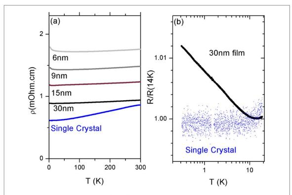
**Figure 3.** Temperature dependence of resistivity for thin films and single crystals of  $Bi_2Ir_2O_7$ . (a) Resistivity versus temperature of a single crystal (blue) and 30–6 nm thick films (black to grey). (b) Semi-log plot of resistance versus temperature of a 30 nm thin film (black) and a single crystal (blue) for the temperature range T = 0.32-20 K. Resistance is normalized by the value at T = 14 K.
