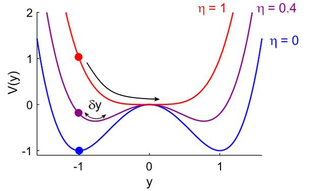
FIG. 1. Normalized Ginzburg-Landau potential  $V(y)$  of the anharmonic lattice dynamics model for various levels of excitation.
