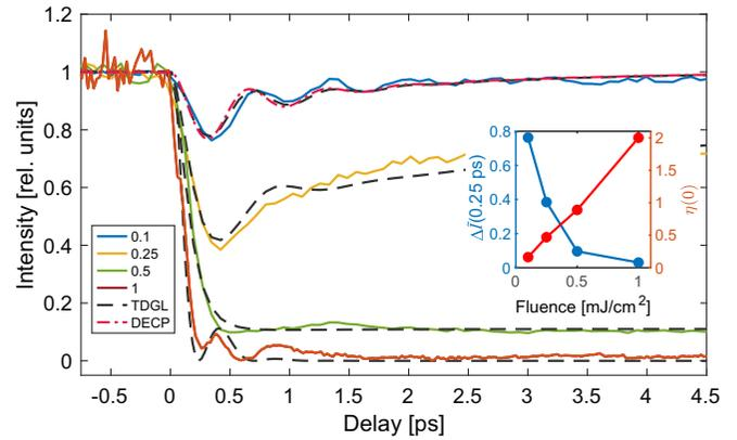
FIG. 6. Time-dependent Ginzburg-Landau model of the dynamics of the order parameter. The solid lines are the time dependence of the structure factor for the (17 $q$ ) reflection as in Fig. 2(a). The dark dashed lines are the solutions to the TDGL for the values reported in Table I. For comparison, the dash-dotted line shows the DECP fit from Fig. 2. The inset shows the fluence dependence of the measured intensity  $\tilde{I}(0.25$  ps) and the fitted value of  $\eta(0)$  (from Table I).
