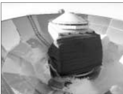
Below: The 2.6m QUaD telescope installed at the South Pole. The secondary mirror is supported by a foam cone to prevent scattering from metallic feed legs from introducing spurious polarized signals.
