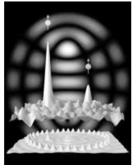
This image shows the electronic signature of a phantom atom (right peak, top) projected from a real atom (left peak, top) inside a nanostructure (elliptical ring) assembled atom by atom. Stanford Prof. Hari Manoharan reported on this "quantum mirage" in the journal Nature while he was working at IBM in 2000.
