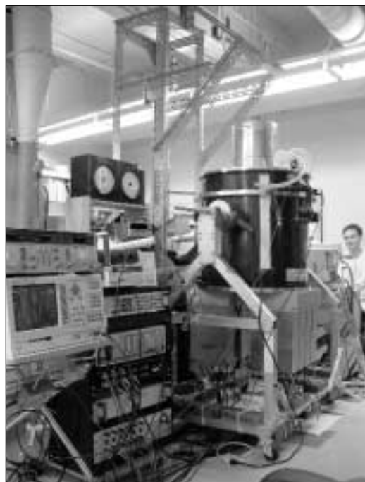
Right: Graduate student James Hinderks testing the QUaD focal plane in its cryostat at Stanford, prior to its shipment to the Pole in October 2004.
