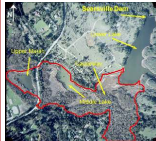
Fig. 4. Map of Searsville Reservoir and its surrounding area. The red outline indicates the approximate original extent of open water.
